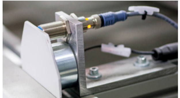
The signals of the sensor and the electromagnet are directly connected to the TBEN-S on the stacker carrier
